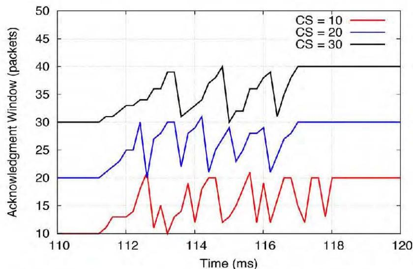
Figure 1. The behavior of transmission window (AW) of CC-CAT
